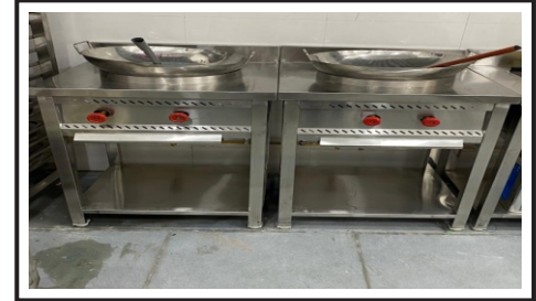
Gas Fryer Burner
